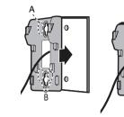
Align and place the telephone base on the wall mount bracket. Slide it down until it clicks securely in place.
