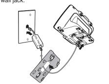
Align and place the wall mount bracket on the standard wall plate.
